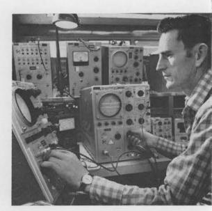
USING ONE OSCILLOSCOPE as a comparator, Alvin Plant (4233-3) calibrates another oscilloscope in electrical standards laboratory. Complete training in secondary standards calibration techniques is part of Electronics Apprenticeship Program. A Sandia employee for six years, Alvin came to the program from Janitor Services Division.
